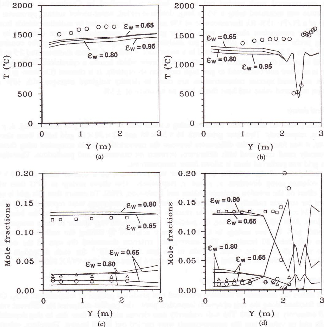
Figure 2. Comparison between predicted (solid lines) and measured (symbols) profiles for different values of the wall emissivity. (a) Temperature profile through port 1.5. (b) Temperature profile through port 3.6. (c) Mole fraction profiles through port 1.5 ( $\square$ :  $\text{CO}_2$ ;  $\Delta$ :  $\text{CO}$ ;  $\circ$ :  $\text{O}_2$ ). (d) Mole fraction profiles through port 2.6 ( $\square$ :  $\text{CO}_2$ ;  $\Delta$ :  $\text{CO}$ ;  $\circ$ :  $\text{O}_2$ )
