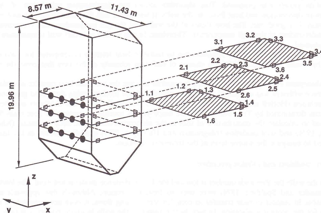
Figure 1. Sketch of the boiler simplified geometry
