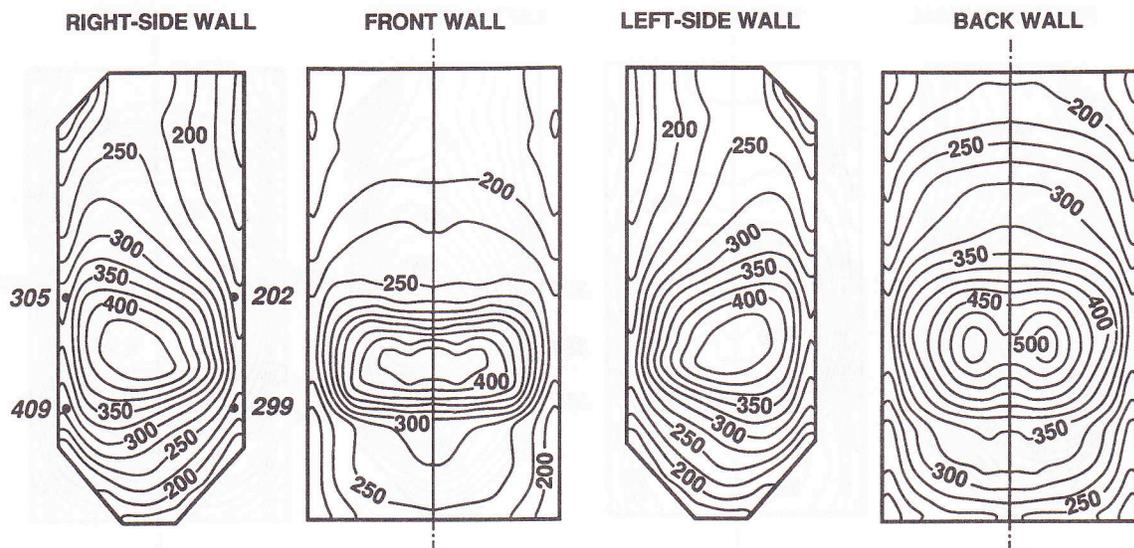
Figure 9. Predicted and measured incident heat fluxes ( $\text{kW m}^{-2}$ ) at partial operation load
