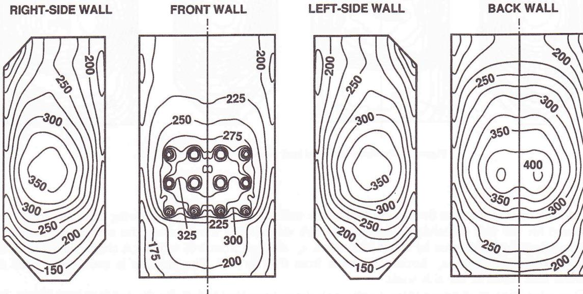
Figure 10. Predicted absorbed heat fluxes ( $\text{kW m}^{-2}$ ) for  $\epsilon_w = 0.65$
