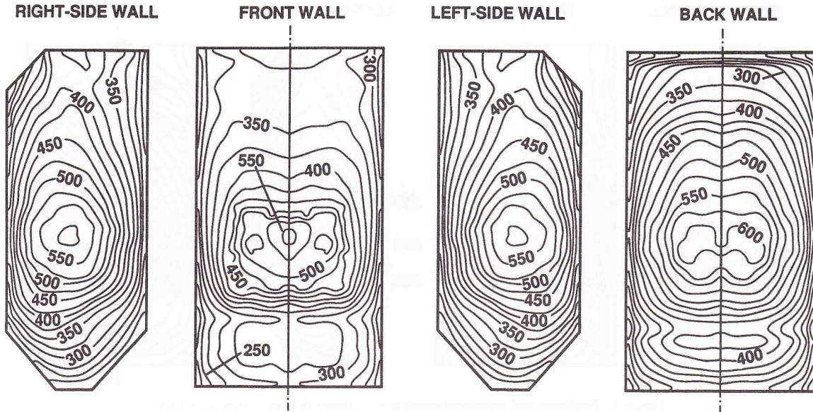
Figure 4. Predicted incident heat fluxes ( $\text{kW m}^{-2}$ ) for  $\epsilon_w = 0.65$  using the same grid for flow and heat transfer calculations
