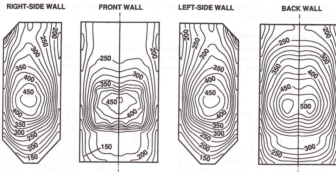
Figure 12. Predicted absorbed heat fluxes ( $\text{kW m}^{-2}$ ) for  $\epsilon_w = 0.95$
