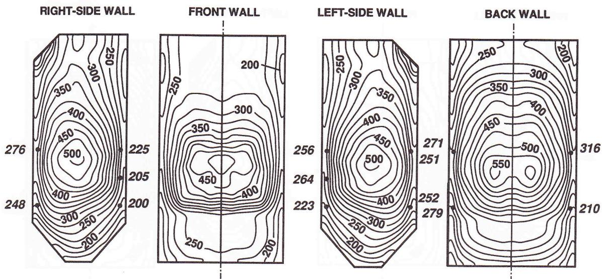
Figure 6. Predicted and measured incident heat fluxes ( $\text{kW m}^{-2}$ ) for  $\epsilon_w = 0.95$
