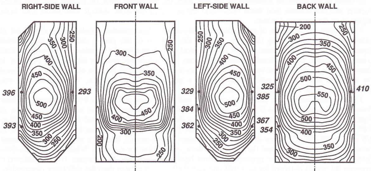
Figure 5. Predicted and measured incident heat fluxes ( $\text{kW m}^{-2}$ ) for  $\epsilon_w = 0.80$
