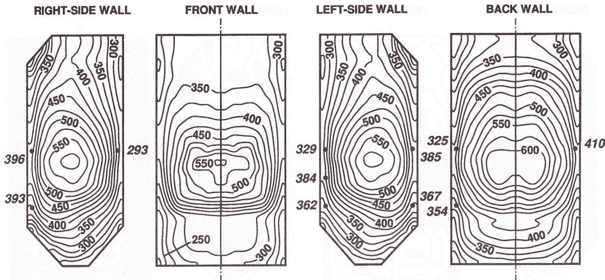
Figure 3. Predicted and measured incident heat fluxes ( $\text{kW m}^{-2}$ ) for  $\epsilon_w = 0.65$
