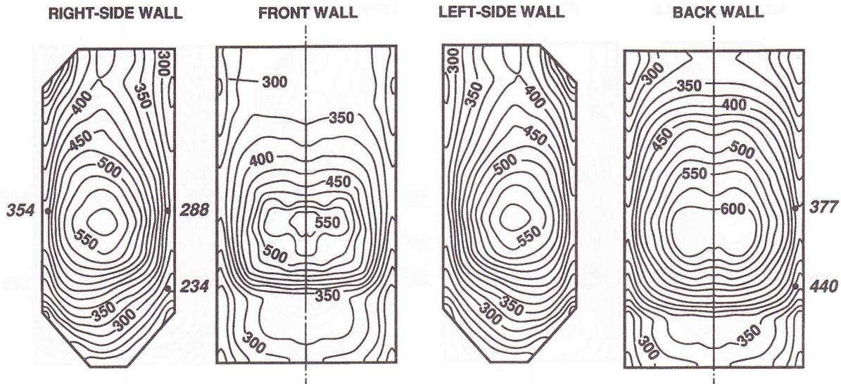
Figure 8. Predicted and measured incident heat fluxes ( $\text{kW m}^{-2}$ ) for 0.75%  $\text{O}_2$  in flue gases
