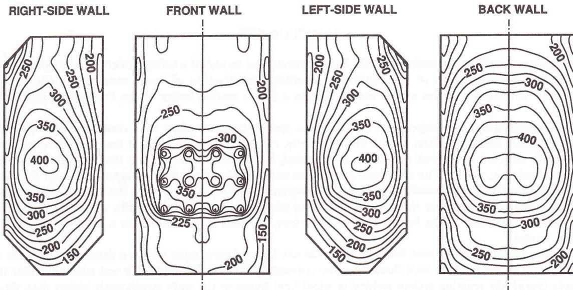
Figure 11. Predicted absorbed heat fluxes ( $\text{kW m}^{-2}$ ) for  $\epsilon_w = 0.80$
