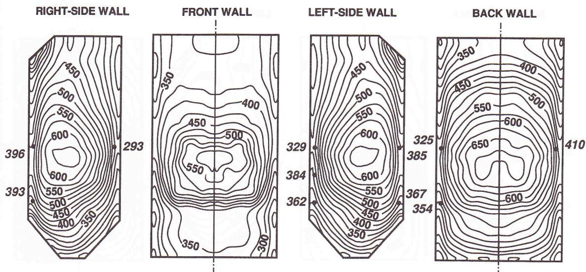
Figure 7. Predicted and measured incident heat fluxes ( $\text{kW m}^{-2}$ ) using the simple chemical reacting system combustion model
