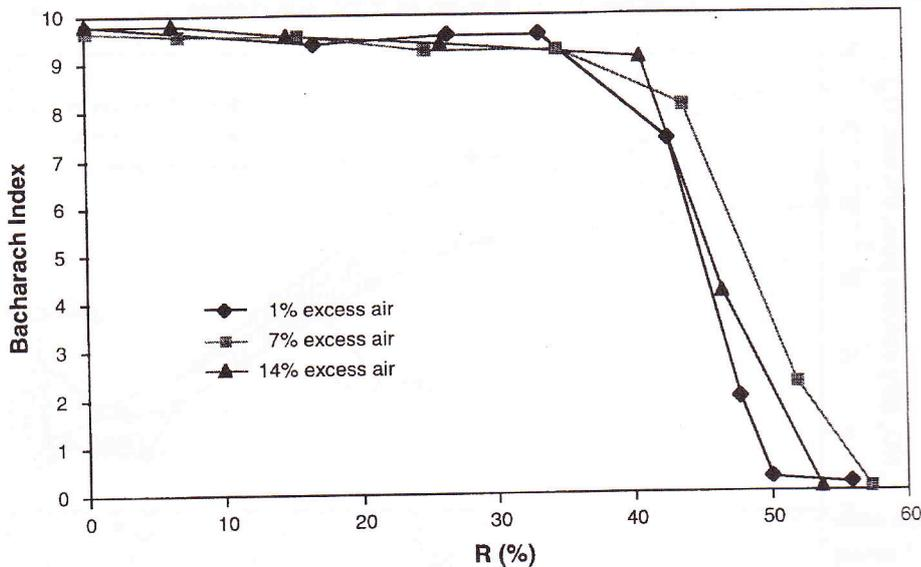
Fig. 6. Effect of FGR on Bacharach Index at three excess air levels, with ethylene
