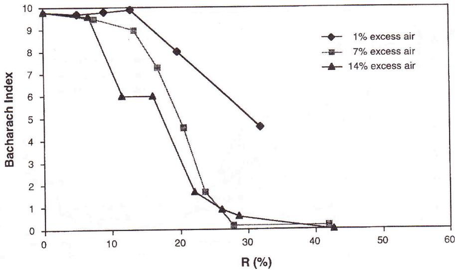
Fig. 5. Effect of FGR on Bacharach Index at three excess air levels, with propane
