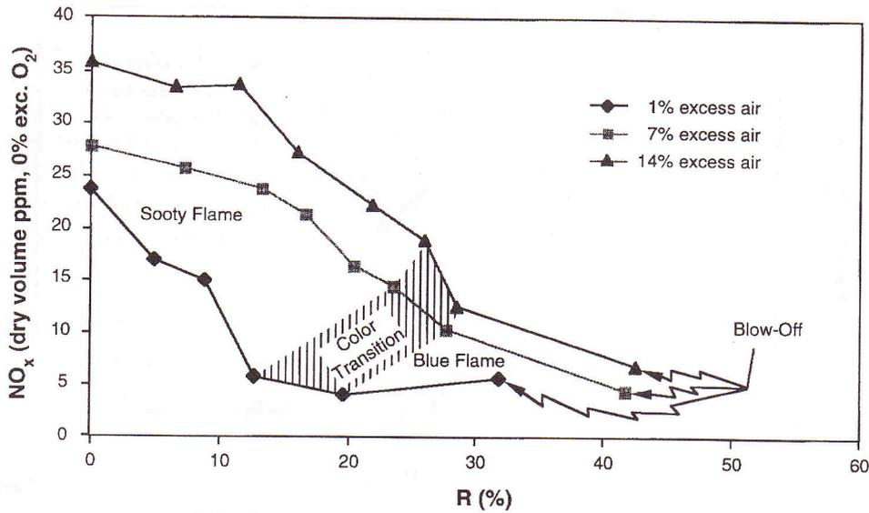
Fig. 3. Effect of FGR on NO<sub>x</sub> emission at three excess air levels, with propane
