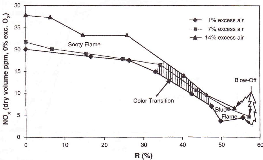
Fig. 4. Effect of FGR on NO<sub>x</sub> emission at three excess air levels, with ethylene
