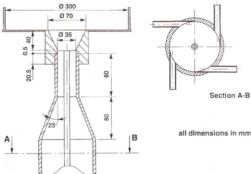
Fig. 2. Schematic of the burner arrangement
