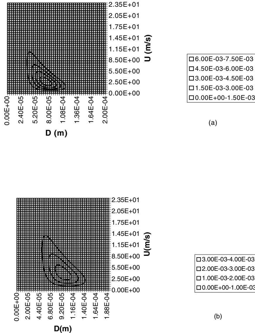
Fig. 7. The effect of the mass flow rate on the droplet size and velocity joint distribution for a plain jet airblast atomiser ( $U_A = 100 \text{ m s}^{-1}$ ,  $d_0 = 2.5 \text{ mm}$ , AFR = 1, fuel: kerosene): (a)  $\dot{M} = 3.0 \times 10^{-3} \text{ kg s}^{-1}$ ; (b)  $\dot{M} = 4.5 \times 10^{-3} \text{ kg s}^{-1}$ .
