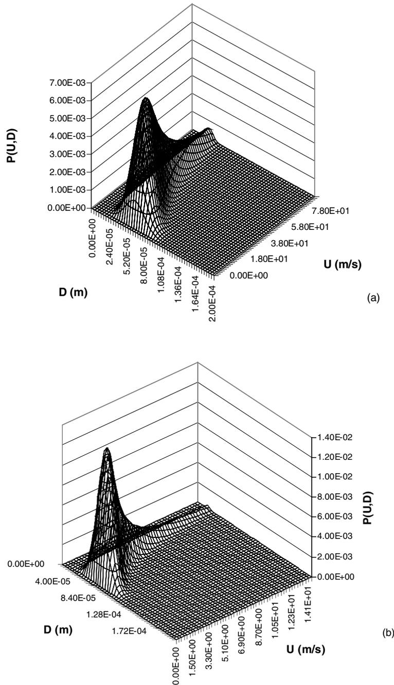
Fig. 2. Droplet size and velocity joint distributions of sprays from: (a) pressure jet atomiser ( $FN = 12.5 \times 10^{-8}$ ,  $d_0 = 3.35 \times 10^{-4}$  m,  $\Delta P_L = 6.9 \times 10^5$  Pa  $m^{-1}$ ,  $\theta = 30^\circ$ , fuel: kerosene); (b) plain jet airblast atomiser ( $U_A = 100$  m  $s^{-1}$ ,  $d_0 = 2.5$  mm, AFR = 1, fuel: kerosene).
