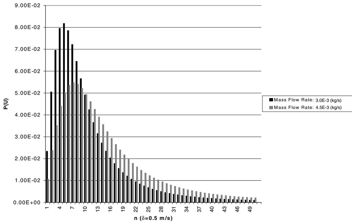
Fig. 6. The effect of the liquid mass flow rate on the droplet velocity distribution for a plain jet airblast atomiser ( $U_A = 100 \text{ m s}^{-1}$ ,  $d_0 = 2.5 \text{ mm}$ , AFR = 1, fuel: kerosene).
