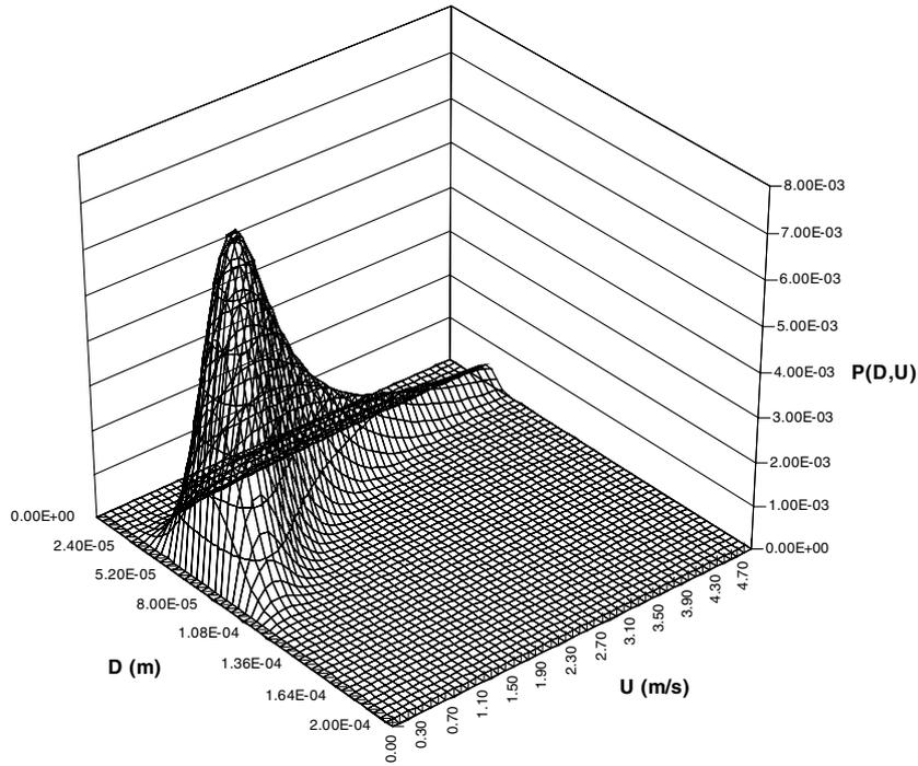
Fig. 1. Droplet size and velocity joint distribution of a spray from a pre-filming airblast atomiser ( $U_A = 100 \text{ m s}^{-1}$ , AFR = 1, fuel: kerosene).
