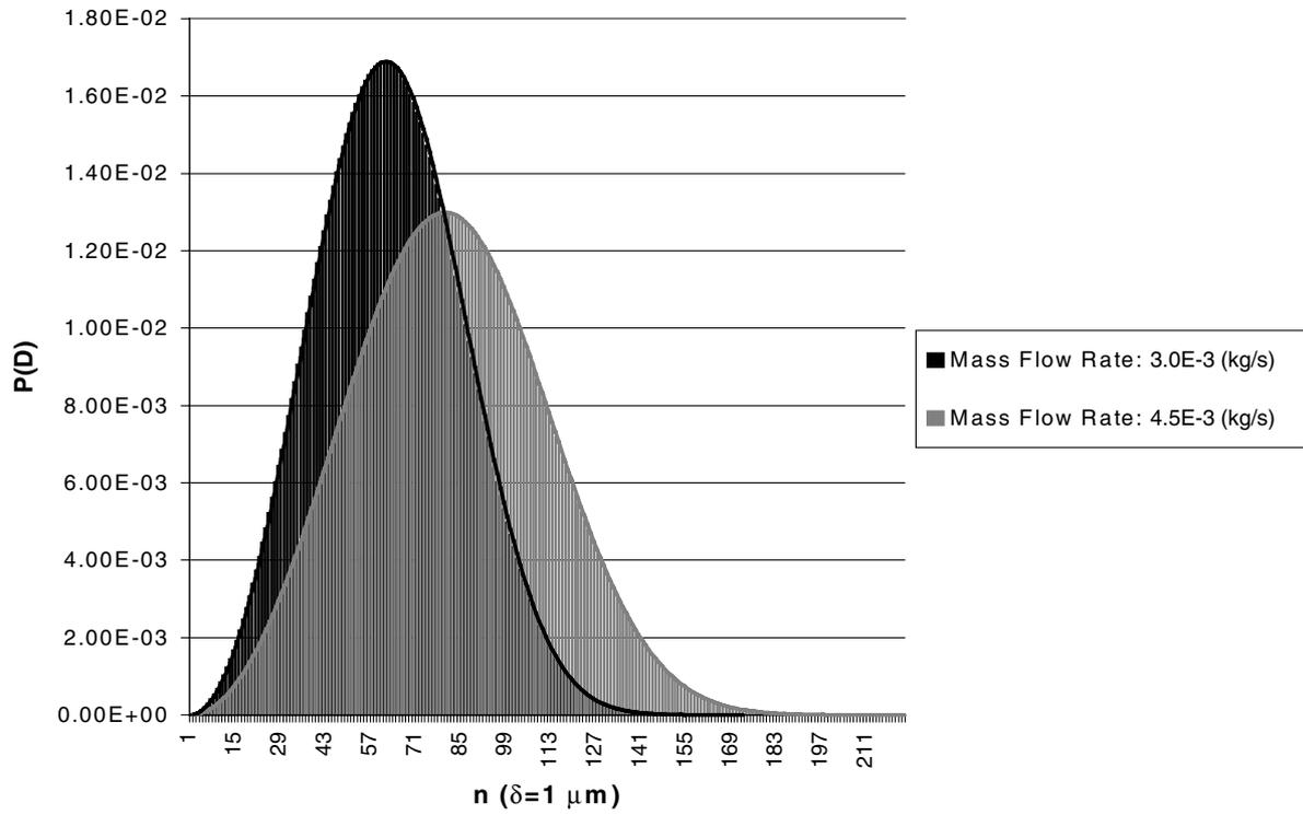
Fig. 5. The effect of the liquid mass flow rate on the droplet size distribution for a plain jet airblast atomiser ( $U_A = 100 \text{ m s}^{-1}$ ,  $d_0 = 2.5 \text{ mm}$ , AFR = 1, fuel: kerosene).
