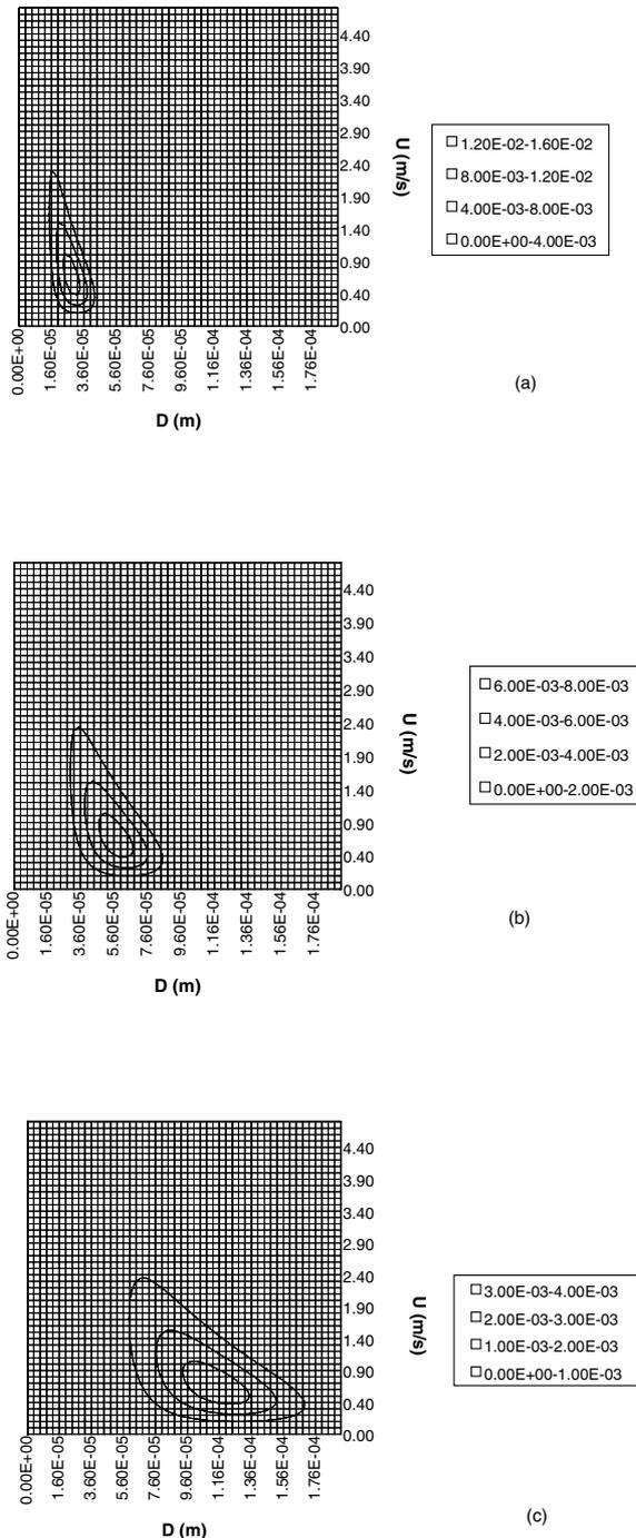
Fig. 4. The effect of the spray fineness—SMD—in a pre-filming airblast atomiser on its velocity distribution ( $\bar{U} = 0.9 \text{ m s}^{-1}$ ): (a) SMD = 30  $\mu\text{m}$ ; (b) SMD = 60  $\mu\text{m}$ ; (c) SMD = 120  $\mu\text{m}$ .
