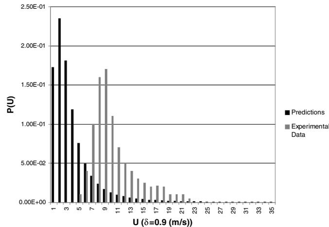
Fig. 3. Comparison of the predicted velocity distribution against experimental data of Presser et al. [20] in a pressure jet atomiser ( $\bar{U} = 7.35 \text{ m s}^{-1}$ ).
