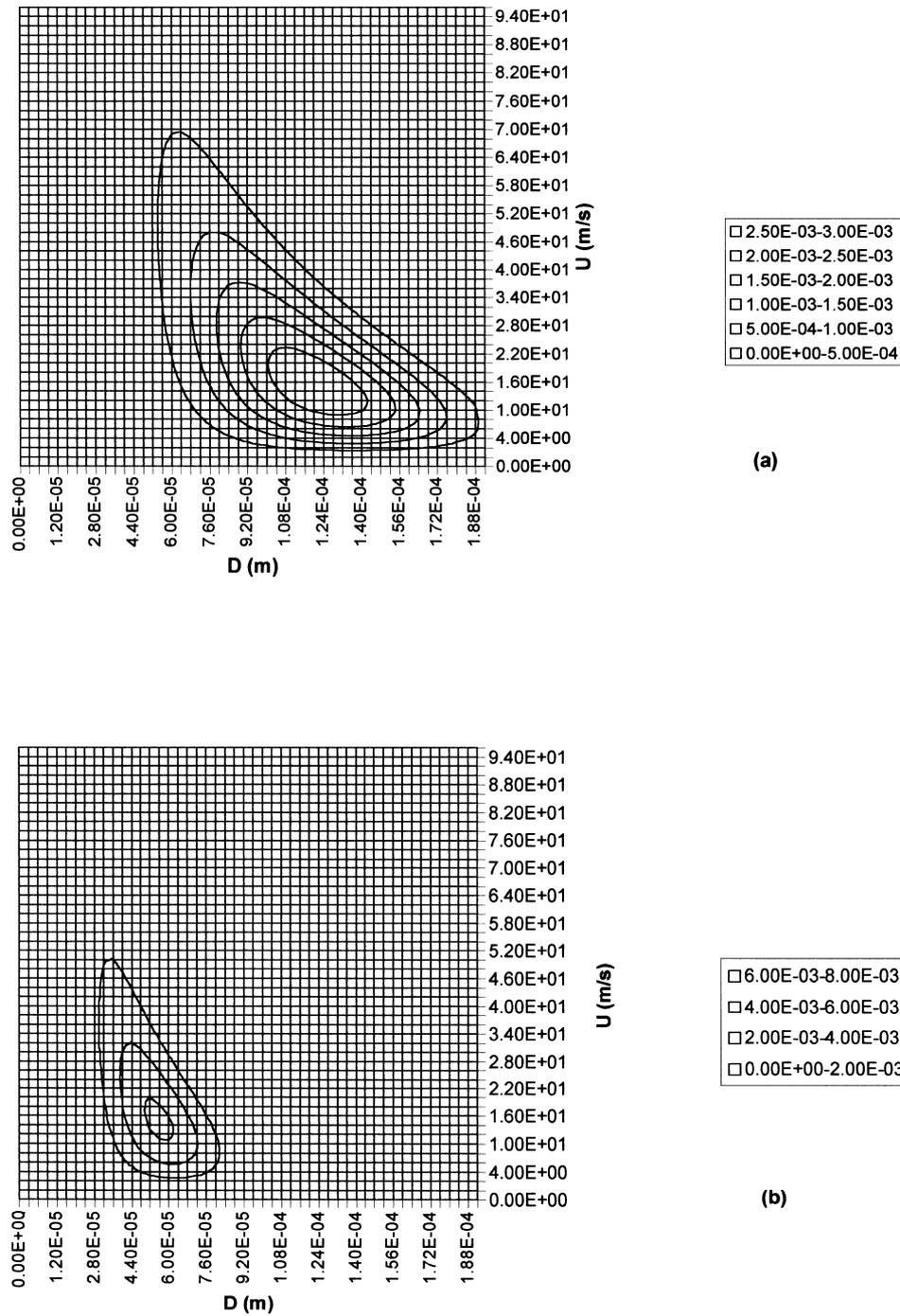
Fig. 8. The effect of fluid properties on the droplet size and velocity joint distribution for a pressure jet atomiser: (a) RFO; (b) water.
